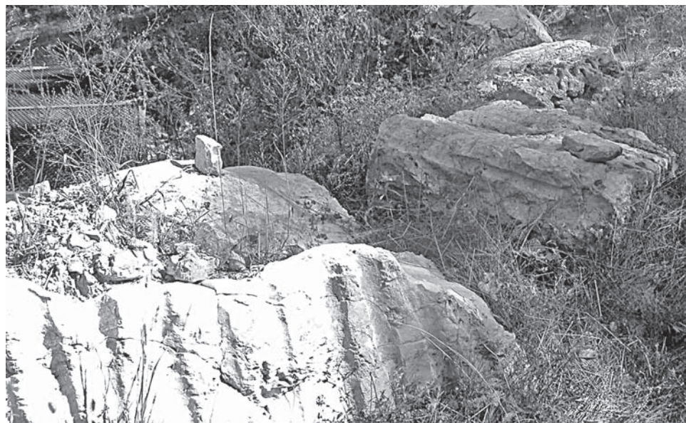
Large blocks of decomposing onyx remain above Onyx Cave near the 125-foot vertical shaft through which they were hoisted to the surface. Drill marks are visible on the nearest block. The onyx was destined for the railroad at Arlington and shipment to a finishing plant in St. Louis. The onyx business collapsed and the Imperial Onyx Company went bankrupt before these blocks could be shipped. Photo by Terry Primas.
